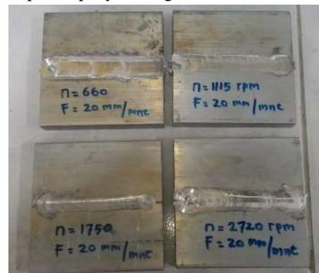
Gambar 3. Hasil Las *Friction Welding*
