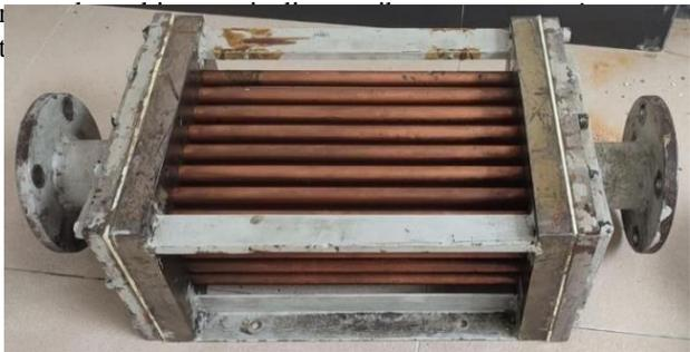
Gambar 4. *Heat exchanger*
