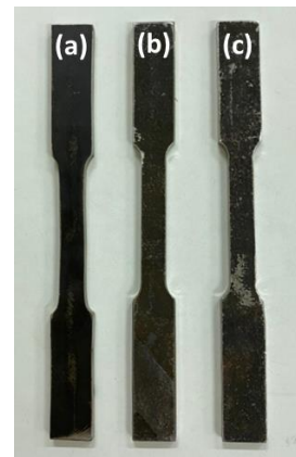
Gambar 3. Spesimen Uji Tarik, (a) Tanpa Perlakuan; (b) Hasil Quenching Media Air; (c) Hasil Quenching Media Air Garam 20 wt.% NaCl
