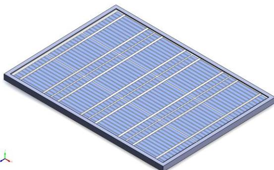
Gambar 2. Rancangan panel surya polycrystalline parafin grafit
