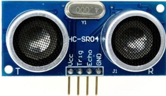
Gambar 3. Sensor Ultrasonic HC-SR04
