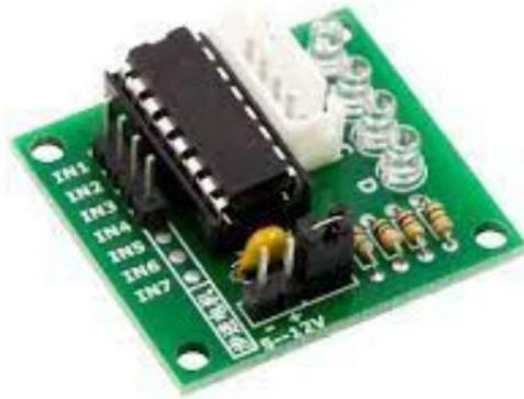
Gambar 5. ULN2003 Modul Driver
