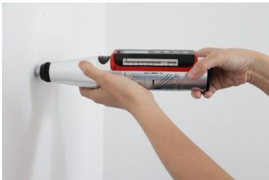
Gambar 2. Hammer Test
