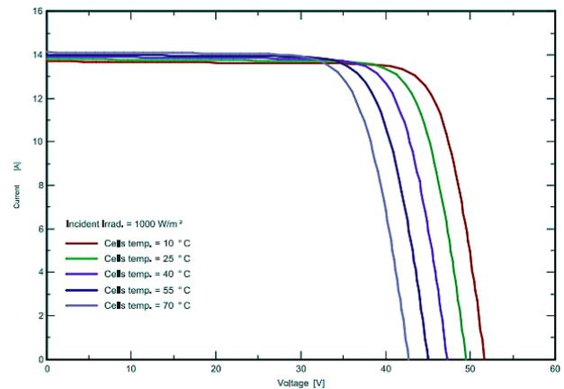
Figure 4. Current and Voltage Versus Temperature
