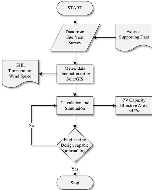
Figure 1. Drafting and Design Flowchart
