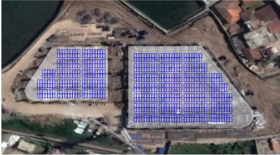
Figure 6. PV Module Layout in FHST Building
