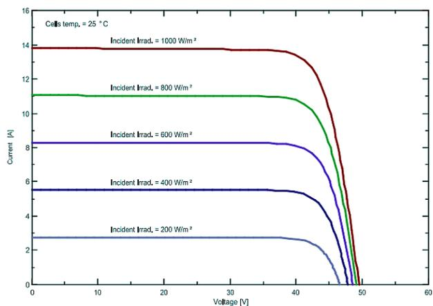
Figure 5. Current and Voltage Versus Irradiation
