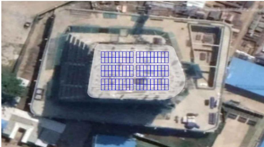
Figure 7. PV Module Layout in Rectorate Building
