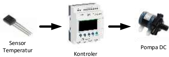
Gambar 4. Diagram blok sistem pendingin photovoltaic
