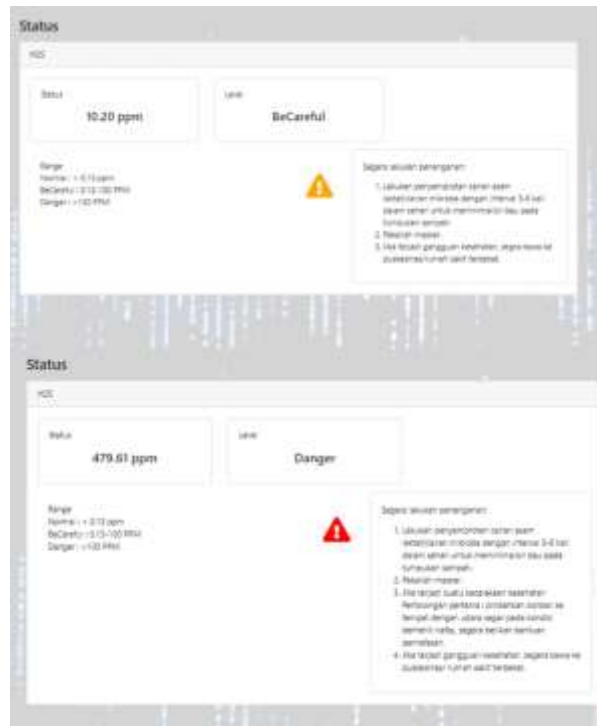
Figure 10. Condition and status of H2S gas on the Dashboard
