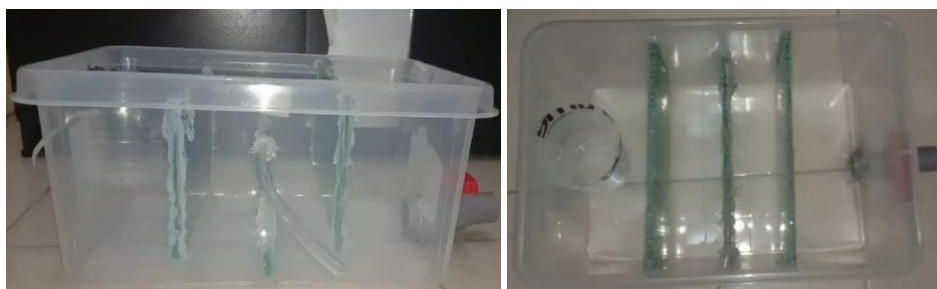
Gambar-3. Grease trap filtrasi bar screen
